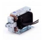
This Solenoid Series has been specifically designed for maximum AC performance, with both the frame and plunger of laminated steel construction, made of special magnetic steel featuring high magnetic permeability and low magnetic losses. Designed to be used in any position, they are able to transform an electric power into an axial pull action.
